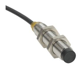
AutomationDirect inductive proximity sensor, tubular, 12mm diameter x 65mm body, bronze-plated brass housing, NPN, N.C. output, 7mm sensing distance, non-flush, 700 Hz switching frequency, IP65 IP66 IP67 IP68 IP69K, pigtail.
