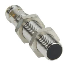
AutomationDirect inductive proximity sensor, tubular, 12mm diameter x 60mm body, bronze-plated brass housing, NPN, N.C. output, 4mm sensing distance, flush, 700 Hz switching frequency, IP65 IP66 IP67 IP68 IP69K, 4-pin M12 quick-disconnect.
