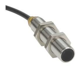
AutomationDirect inductive proximity sensor, tubular, 12mm diameter x 65mm body, bronze-plated brass housing, NPN, N.C. output, 4mm sensing distance, flush, 700 Hz switching frequency, IP65 IP66 IP67 IP68 IP69K, pigtail.
