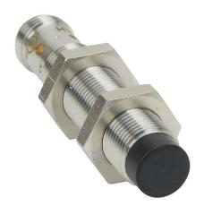
AutomationDirect inductive proximity sensor, tubular, 12mm diameter x 60mm body, bronze-plated brass housing, PNP, N.O. output, 7mm sensing distance, non-flush, 700 Hz switching frequency, IP65 IP66 IP67 IP68 IP69K, 4-pin M12 quick-disconnect.
