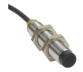
AutomationDirect inductive proximity sensor, tubular, 12mm diameter x 65mm body, bronze-plated brass housing, PNP, N.O. output, 7mm sensing distance, non-flush, 700 Hz switching frequency, IP65 IP66 IP67 IP68 IP69K, pigtail.
