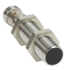
AutomationDirect inductive proximity sensor, tubular, 12mm diameter x 60mm body, bronze-plated brass housing, PNP, N.O. output, 4mm sensing distance, flush, 700 Hz switching frequency, IP65 IP66 IP67 IP68 IP69K, 4-pin M12 quick-disconnect.
