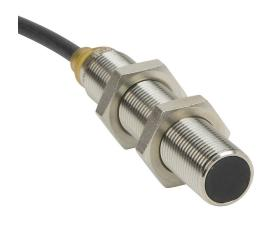
AutomationDirect inductive proximity sensor, tubular, 12mm diameter x 65mm body, bronze-plated brass housing, PNP, N.O. output, 4mm sensing distance, flush, 700 Hz switching frequency, IP65 IP66 IP67 IP68 IP69K, pigtail.
