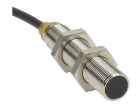
AutomationDirect inductive proximity sensor, tubular, 12mm diameter x 65mm body, bronze-plated brass housing, PNP, N.O. output, 4mm sensing distance, flush, 700 Hz switching frequency, IP65 IP66 IP67 IP68 IP69K, pigtail.
