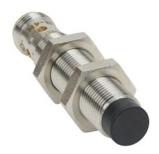
AutomationDirect inductive proximity sensor, tubular, 12mm diameter x 60mm body, bronze-plated brass housing, NPN, N.O. output, 7mm sensing distance, non-flush, 700 Hz switching frequency, IP65 IP66 IP67 IP68 IP69K, 4-pin M12 quick-disconnect.
