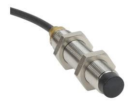
AutomationDirect inductive proximity sensor, tubular, 12mm diameter x 65mm body, bronze-plated brass housing, NPN, N.O. output, 7mm sensing distance, non-flush, 700 Hz switching frequency, IP65 IP66 IP67 IP68 IP69K, pigtail.
