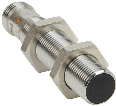
AutomationDirect inductive proximity sensor, tubular, 12mm diameter x 60mm body, bronze-plated brass housing, NPN, N.O. output, 4mm sensing distance, flush, 700 Hz switching frequency, IP65 IP66 IP67 IP68 IP69K, 4-pin M12 quick-disconnect.
