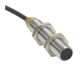
AutomationDirect inductive proximity sensor, tubular, 12mm diameter x 65mm body, bronze-plated brass housing, NPN, N.O. output, 4mm sensing distance, flush, 700 Hz switching frequency, IP65 IP66 IP67 IP68 IP69K, pigtail.
