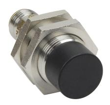
AutomationDirect inductive proximity sensor, tubular, 18mm diameter x 45mm body, bronze-plated brass housing, PNP, N.C. output, 12mm sensing distance, non-flush, 300 Hz switching frequency, IP65 IP66 IP67 IP68 IP69K, 4-pin M12 quick-disconnect.
