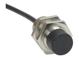
AutomationDirect inductive proximity sensor, tubular, 18mm diameter x 45mm body, bronze-plated brass housing, PNP, N.C. output, 12mm sensing distance, non-flush, 300 Hz switching frequency, IP65 IP66 IP67 IP68 IP69K, pigtail.
