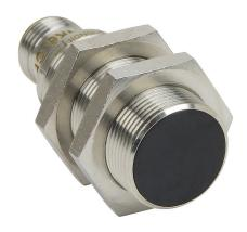
AutomationDirect inductive proximity sensor, tubular, 18mm diameter x 45mm body, bronze-plated brass housing, PNP, N.C. output, 8mm sensing distance, flush, 400 Hz switching frequency, IP65 IP66 IP67 IP68 IP69K, 4-pin M12 quick-disconnect.
