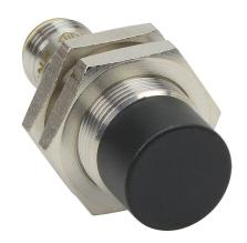
AutomationDirect inductive proximity sensor, tubular, 18mm diameter x 45mm body, bronze-plated brass housing, NPN, N.C. output, 12mm sensing distance, non-flush, 300 Hz switching frequency, IP65 IP66 IP67 IP68 IP69K, 4-pin M12 quick-disconnect.
