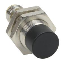
AutomationDirect inductive proximity sensor, tubular, 18mm diameter x 45mm body, bronze-plated brass housing, NPN, N.C. output, 12mm sensing distance, non-flush, 300 Hz switching frequency, IP65 IP66 IP67 IP68 IP69K, 4-pin M12 quick-disconnect.
