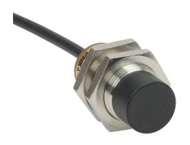
AutomationDirect inductive proximity sensor, tubular, 18mm diameter x 45mm body, bronze-plated brass housing, NPN, N.C. output, 12mm sensing distance, non-flush, 300 Hz switching frequency, IP65 IP66 IP67 IP68 IP69K, pigtail.
