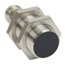
AutomationDirect inductive proximity sensor, tubular, 18mm diameter x 45mm body, bronze-plated brass housing, NPN, N.C. output, 8mm sensing distance, flush, 400 Hz switching frequency, IP65 IP66 IP67 IP68 IP69K, 4-pin M12 quick-disconnect.
