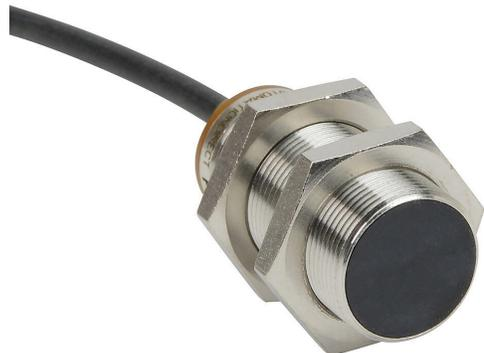
AutomationDirect inductive proximity sensor, tubular, 18mm diameter x 45mm body, bronze-plated brass housing, NPN, N.C. output, 8mm sensing distance, flush, 400 Hz switching frequency, IP65 IP66 IP67 IP68 IP69K, pigtail.
