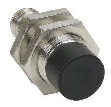
AutomationDirect inductive proximity sensor, tubular, 18mm diameter x 45mm body, bronze-plated brass housing, PNP, N.O. output, 12mm sensing distance, non-flush, 300 Hz switching frequency, IP65 IP66 IP67 IP68 IP69K, 4-pin M12 quick-disconnect.
