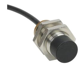
AutomationDirect inductive proximity sensor, tubular, 18mm diameter x 45mm body, bronze-plated brass housing, PNP, N.O. output, 12mm sensing distance, non-flush, 300 Hz switching frequency, IP65 IP66 IP67 IP68 IP69K, pigtail.
