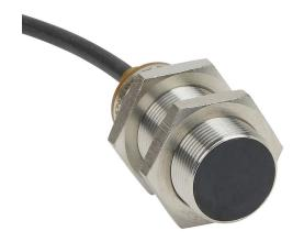
AutomationDirect inductive proximity sensor, tubular, 18mm diameter x 45mm body, bronze-plated brass housing, PNP, N.O. output, 8mm sensing distance, flush, 400 Hz switching frequency, IP65 IP66 IP67 IP68 IP69K, pigtail.
