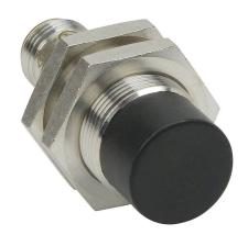
AutomationDirect inductive proximity sensor, tubular, 18mm diameter x 45mm body, bronze-plated brass housing, NPN, N.O. output, 12mm sensing distance, non-flush, 300 Hz switching frequency, IP65 IP66 IP67 IP68 IP69K, 4-pin M12 quick-disconnect.
