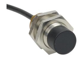
AutomationDirect inductive proximity sensor, tubular, 18mm diameter x 45mm body, bronze-plated brass housing, NPN, N.O. output, 12mm sensing distance, non-flush, 300 Hz switching frequency, IP65 IP66 IP67 IP68 IP69K, pigtail.
