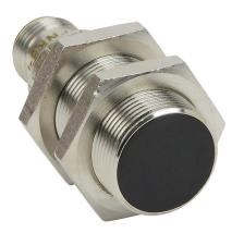
AutomationDirect inductive proximity sensor, tubular, 18mm diameter x 45mm body, bronze-plated brass housing, NPN, N.O. output, 8mm sensing distance, flush, 400 Hz switching frequency, IP65 IP66 IP67 IP68 IP69K, 4-pin M12 quick-disconnect.
