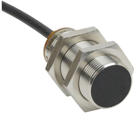
AutomationDirect inductive proximity sensor, tubular, 18mm diameter x 45mm body, bronze-plated brass housing, NPN, N.O. output, 8mm sensing distance, flush, 400 Hz switching frequency, IP65 IP66 IP67 IP68 IP69K, pigtail.
