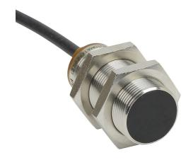
AutomationDirect inductive proximity sensor, tubular, 18mm diameter x 45mm body, bronze-plated brass housing, NPN, N.O. output, 8mm sensing distance, flush, 400 Hz switching frequency, IP65 IP66 IP67 IP68 IP69K, pigtail.
