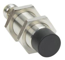
AutomationDirect inductive proximity sensor, tubular, 18mm diameter x 60mm body, bronze-plated brass housing, PNP, N.C. output, 12mm sensing distance, non-flush, 300 Hz switching frequency, IP65 IP66 IP67 IP68 IP69K, 4-pin M12 quick-disconnect.
