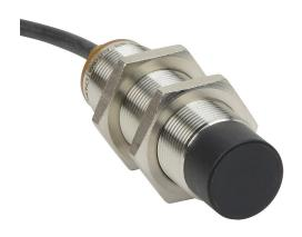
AutomationDirect inductive proximity sensor, tubular, 18mm diameter x 65mm body, bronze-plated brass housing, PNP, N.C. output, 12mm sensing distance, non-flush, 300 Hz switching frequency, IP65 IP66 IP67 IP68 IP69K, pigtail.
