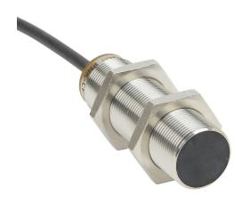
AutomationDirect inductive proximity sensor, tubular, 18mm diameter x 65mm body, bronze-plated brass housing, PNP, N.C. output, 8mm sensing distance, flush, 400 Hz switching frequency, IP65 IP66 IP67 IP68 IP69K, pigtail.
