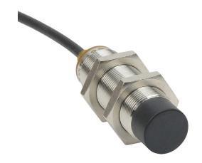
AutomationDirect inductive proximity sensor, tubular, 18mm diameter x 65mm body, bronze-plated brass housing, NPN, N.C. output, 12mm sensing distance, non-flush, 300 Hz switching frequency, IP65 IP66 IP67 IP68 IP69K, pigtail.
