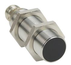
AutomationDirect inductive proximity sensor, tubular, 18mm diameter x 60mm body, bronze-plated brass housing, NPN, N.C. output, 8mm sensing distance, flush, 400 Hz switching frequency, IP65 IP66 IP67 IP68 IP69K, 4-pin M12 quick-disconnect.
