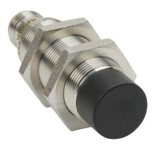
AutomationDirect inductive proximity sensor, tubular, 18mm diameter x 60mm body, bronze-plated brass housing, PNP, N.O. output, 12mm sensing distance, non-flush, 300 Hz switching frequency, IP65 IP66 IP67 IP68 IP69K, 4-pin M12 quick-disconnect.
