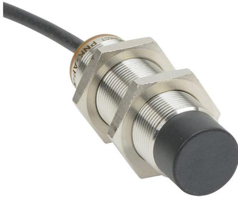
AutomationDirect inductive proximity sensor, tubular, 18mm diameter x 65mm body, bronze-plated brass housing, PNP, N.O. output, 12mm sensing distance, non-flush, 300 Hz switching frequency, IP65 IP66 IP67 IP68 IP69K, pigtail.
