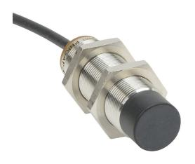
AutomationDirect inductive proximity sensor, tubular, 18mm diameter x 65mm body, bronze-plated brass housing, PNP, N.O. output, 12mm sensing distance, non-flush, 300 Hz switching frequency, IP65 IP66 IP67 IP68 IP69K, pigtail.
