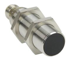
AutomationDirect inductive proximity sensor, tubular, 18mm diameter x 60mm body, bronze-plated brass housing, PNP, N.O. output, 8mm sensing distance, flush, 400 Hz switching frequency, IP65 IP66 IP67 IP68 IP69K, 4-pin M12 quick-disconnect.
