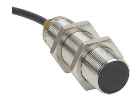
AutomationDirect inductive proximity sensor, tubular, 18mm diameter x 65mm body, bronze-plated brass housing, PNP, N.O. output, 8mm sensing distance, flush, 400 Hz switching frequency, IP65 IP66 IP67 IP68 IP69K, pigtail.
