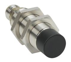
AutomationDirect inductive proximity sensor, tubular, 18mm diameter x 60mm body, bronze-plated brass housing, NPN, N.O. output, 12mm sensing distance, non-flush, 300 Hz switching frequency, IP65 IP66 IP67 IP68 IP69K, 4-pin M12 quick-disconnect.
