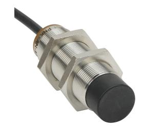
AutomationDirect inductive proximity sensor, tubular, 18mm diameter x 65mm body, bronze-plated brass housing, NPN, N.O. output, 12mm sensing distance, non-flush, 300 Hz switching frequency, IP65 IP66 IP67 IP68 IP69K, pigtail.
