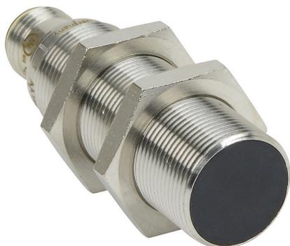
AutomationDirect inductive proximity sensor, tubular, 18mm diameter x 60mm body, bronze-plated brass housing, NPN, N.O. output, 8mm sensing distance, flush, 400 Hz switching frequency, IP65 IP66 IP67 IP68 IP69K, 4-pin M12 quick-disconnect.
