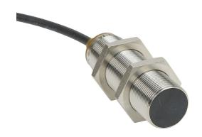
AutomationDirect inductive proximity sensor, tubular, 18mm diameter x 65mm body, bronze-plated brass housing, NPN, N.O. output, 8mm sensing distance, flush, 400 Hz switching frequency, IP65 IP66 IP67 IP68 IP69K, pigtail.
