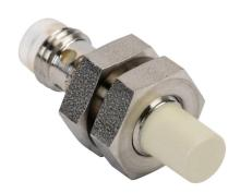
ProSense inductive proximity sensor, tubular, 8mm diameter x 30mm body, stainless steel housing, PNP, N.C. output, 6mm sensing distance, non-flush, 800 Hz switching frequency, IP65 IP66 IP67 IP68 IP69K, 3-pin M8 quick-disconnect.
