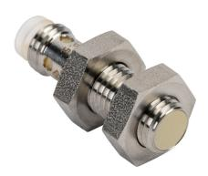
ProSense inductive proximity sensor, tubular, 8mm diameter x 30mm body, stainless steel housing, PNP, N.C. output, 3mm sensing distance, flush, 1.5 kHz switching frequency, IP65 IP66 IP67 IP68 IP69K, 3-pin M8 quick-disconnect.
