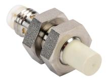
ProSense inductive proximity sensor, tubular, 8mm diameter x 30mm body, stainless steel housing, PNP, N.O. output, 6mm sensing distance, non-flush, 800 Hz switching frequency, IP65 IP66 IP67 IP68 IP69K, 3-pin M8 quick-disconnect.
