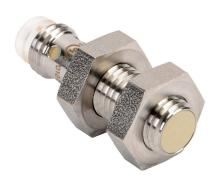
ProSense inductive proximity sensor, tubular, 8mm diameter x 30mm body, stainless steel housing, PNP, N.O. output, 3mm sensing distance, flush, 1.5 kHz switching frequency, IP65 IP66 IP67 IP68 IP69K, 3-pin M8 quick-disconnect.
