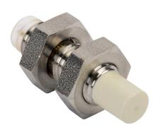
ProSense inductive proximity sensor, tubular, 8mm diameter x 30mm body, stainless steel housing, NPN, N.O. output, 6mm sensing distance, non-flush, 800 Hz switching frequency, IP65 IP66 IP67 IP68 IP69K, 3-pin M8 quick-disconnect.
