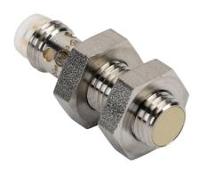
ProSense inductive proximity sensor, tubular, 8mm diameter x 30mm body, stainless steel housing, NPN, N.O. output, 3mm sensing distance, flush, 1.5 kHz switching frequency, IP65 IP66 IP67 IP68 IP69K, 3-pin M8 quick-disconnect.
