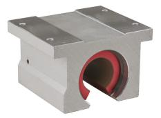
PBC Simplicity series single pillow block, plain bearing, 3.38in overall length, PTFE, 1-1/4in inside diameter, aluminum housing, 0.0015in running clearance. For use with 1-1/4in diameter PBC shafts.
