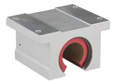
PBC Simplicity series single pillow block, plain bearing, 2.63in overall length, PTFE, 1in inside diameter, aluminum housing, 0.0005in running clearance. For use with 1in diameter PBC shafts.
