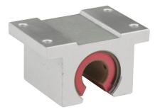
PBC Simplicity series single pillow block, plain bearing, 1.75in overall length, PTFE, 5/8in inside diameter, aluminum housing, 0.0015in running clearance. For use with 5/8in diameter PBC shafts.
