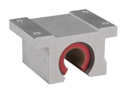
PBC Simplicity series single pillow block, plain bearing, 1.5in overall length, PTFE, 1/2in inside diameter, aluminum housing, 0.0005in running clearance. For use with 1/2in diameter PBC shafts.
