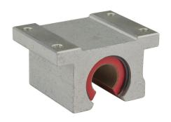
PBC Simplicity series single pillow block, plain bearing, 1.5in overall length, PTFE, 1/2in inside diameter, aluminum housing, 0.0015in running clearance. For use with 1/2in diameter PBC shafts.
