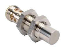
ProSense inductive proximity sensor, tubular, 12mm diameter x 45mm body, stainless steel housing, PNP, N.O. output, 6mm sensing distance, non-flush, 250 Hz switching frequency, IP65 IP66 IP67 IP68 IP69K, 4-pin M12 quick-disconnect.
